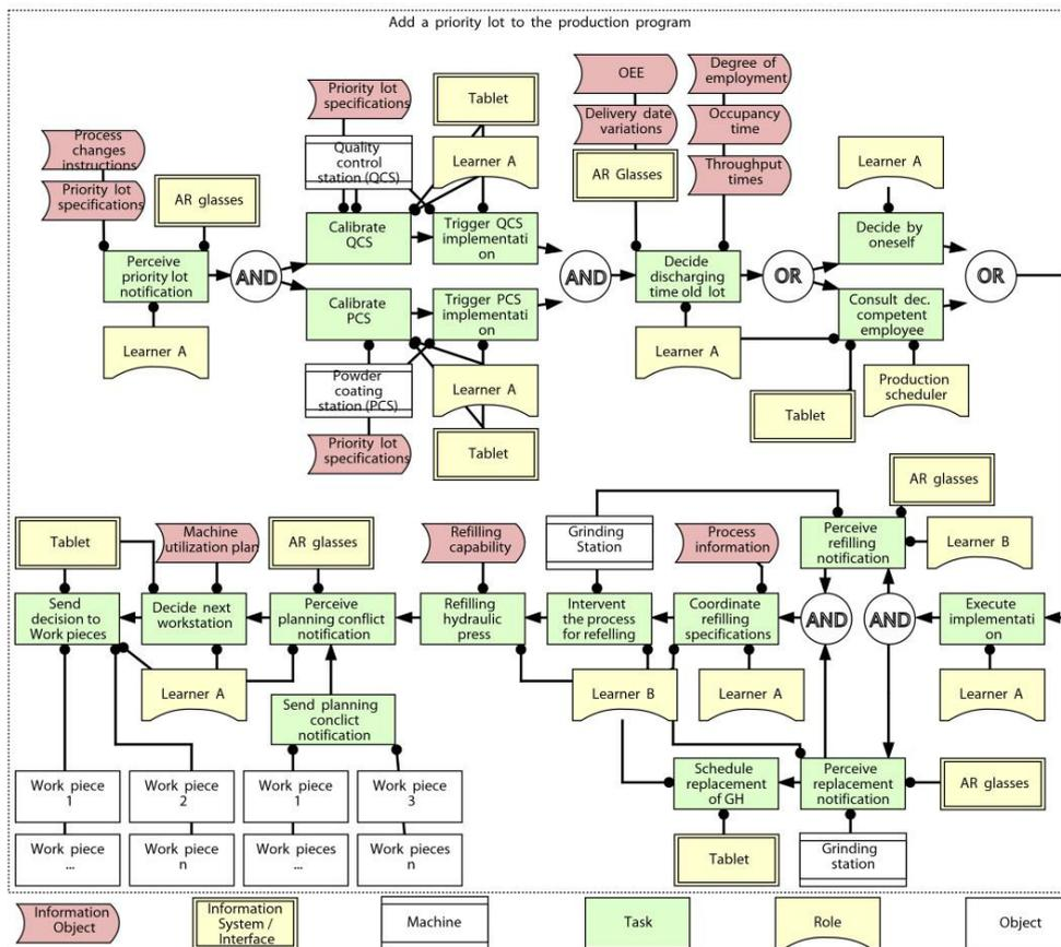
Fig. 3. Process model scenario “Add a priority lot to the production program”.
